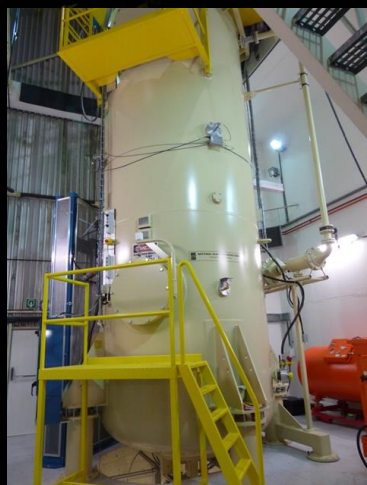
MONNET, Tandem accelerator based fast neutron source
