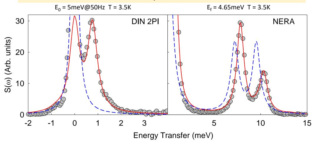
LLW CEF parameters: x = 0.0066 W = 0.03374 meV (blue line) + Molecular Field:  $H_z = 0.18 \text{meV} (2.1T)$  (red line)
