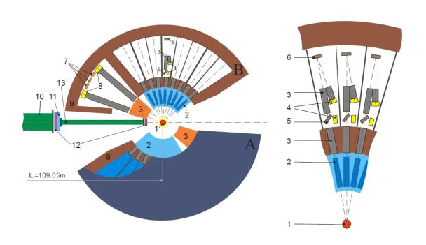
**Figure 3.** The main part of the NERA spectrometer: 1 - sample, 2 - Be-filters, 3 - collimators, 4 - He-3 detectors (INS and QENS), 5 - PG analysers (INS), 6 - single crystal analysers (QENS), 7 - detectors for high intensity diffraction, 8 - diffraction detectors with a good collimation, 9 - spectrometer shielding, 10 - Ni-coated mirror neutron guide in a vacuum tube, 11 - incident beam monitor, 12 - diaphragms, 13 - vacuum neutron guide.
