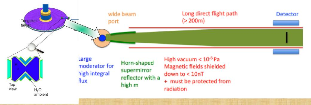
ESS: European Spallation Source. $n - \overline{n}$  is the largest experiment currently considered at ESS (USA-Europe collaboration with over 50 main participants from over 20 universities/institutes. Extensive improvement of parameters of the previous experiment. An expected gain of 2-3 orders of magnitude.
