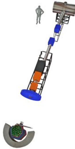
Fig. 35. Layout of the new inelastic neutron scattering spectrometer with inverse geometry on beamline 2 of the IBR-2 reactor.
