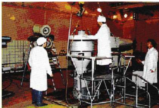
Assembling of multiplying system at FKBN-2
