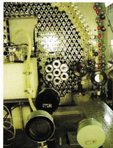
*Multi-element laser channel in the laser block of the reactor-laser system of Rig B*
