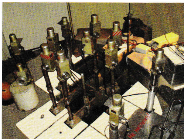
Reactor room. A view of the MAKET CF head assembly
