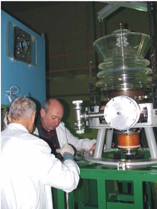
Fig.5. Assembling of the electron gun.
