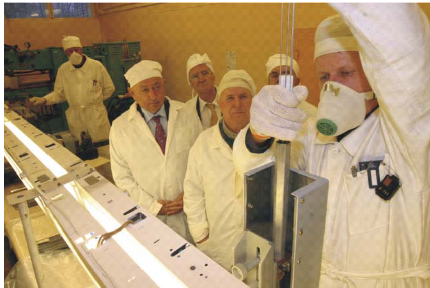
Fig.8. Assembling of fuel elements into fuel assemblies for the IBR-2M reactor.
