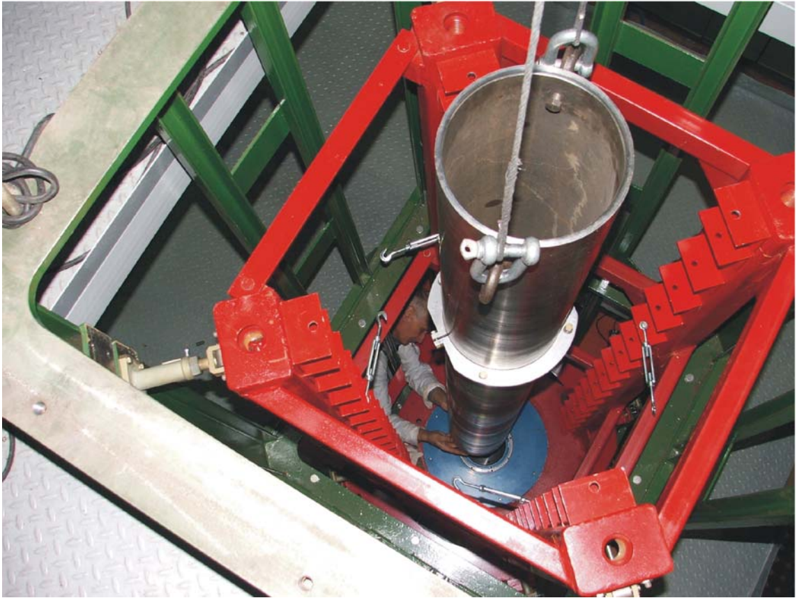
Fig.4. Assembling of the focusing solenoid.
