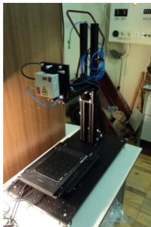
*Fig. 1-III-19. Two-coordinate laser vibrometer.*
