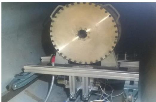
**Fig. 1-IV-10.** A platform with a detector mounted on the position adjustment mechanism for moving in the horizontal and vertical directions.
