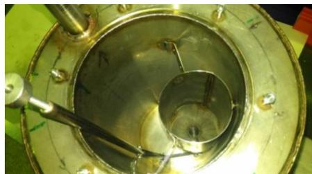
*Fig. 1-IV-1. A device for nitrogen-free charging of frozen pellets into the CM202 chamber.*
