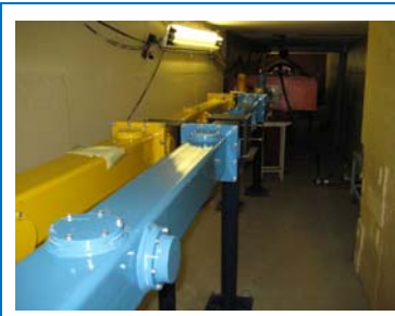
Fig. 4. First sections of the curved neutron guides for EPSILON (yellow) and SKAT (blue).
