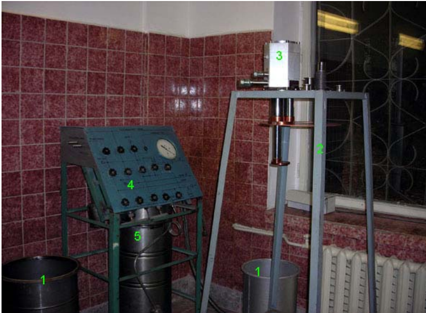
Fig. 8. A test cryostat of the cryogenic stand (1 – cryostat, 2 – cryostat trestle, 3 – cold head, 4 – control panel of the gas circulation system, 5 – He-3 storage tank).
