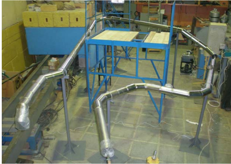
Fig. 2. Mounting of the cryogenic transport tube.
