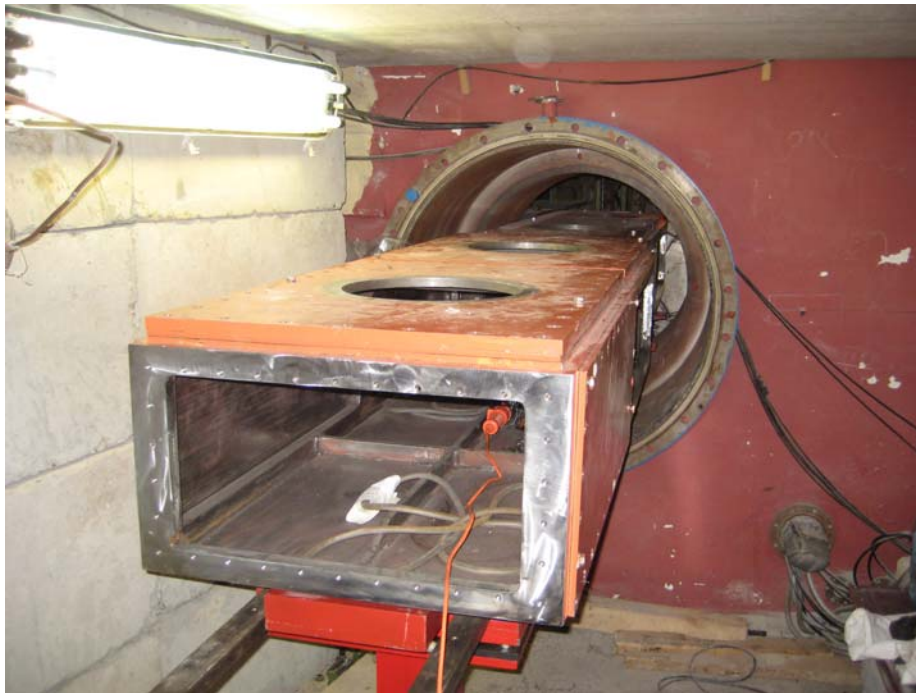
Fig. 13. The head part of the splitter of beam 7 of the IBR-2M reactor for the neutron guide system of the EPSILON (7A-1), SKAT (7A-2) and NERA (7B) diffractometers. The installation of the splitter is carried out within the framework of the BMBF project on modernization of the neutron guide system of the EPSILON and SKAT diffractometers on beam 7A of the IBR-2M reactor.
