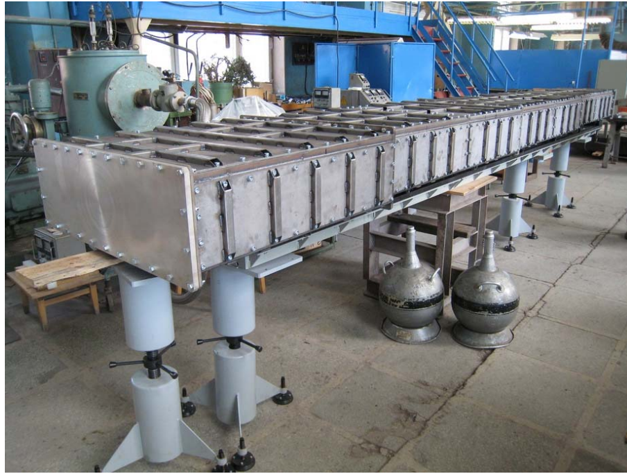
Fig. 11. The head part of the GRAINS reflectometer.
